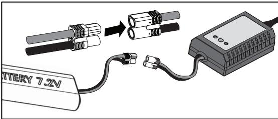
The vehicle battery charger produces 2000 milliAmps (2 Amps) per hour. Divide the mAh capacity on the label of a battery by 2000 to know how long battery charging will require. For example, an 1800mAh battery requires 0.9 hours (54 minutes) to charge.
